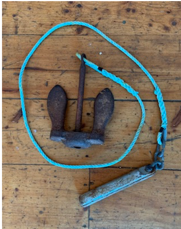
Figure 4. Anchor with 10-foot leash and an anchor leash weight.
