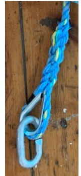
Figure 2. Eye splice reinforced with a thimble.
